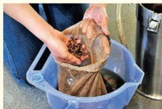
Check the sludge on the filter media (for odor & viscosity).
