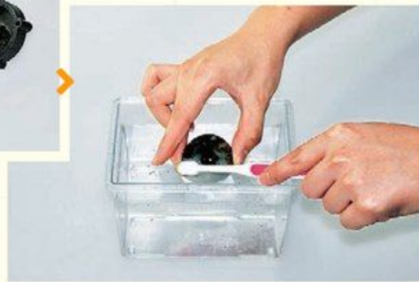
Remove the front casing to take out the impeller. It is very dirty as you can see in the photo.
