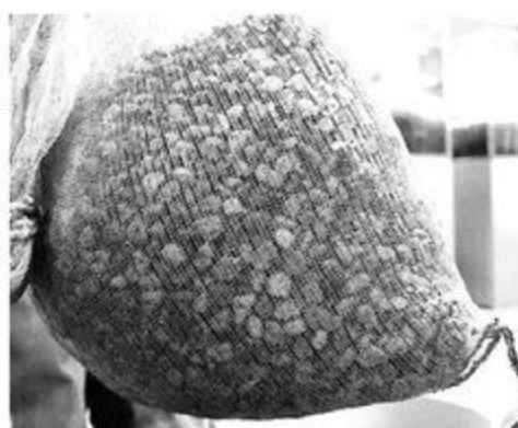
Select the net with coarse mesh but not too coarse to allow the filter media to penetrate.
