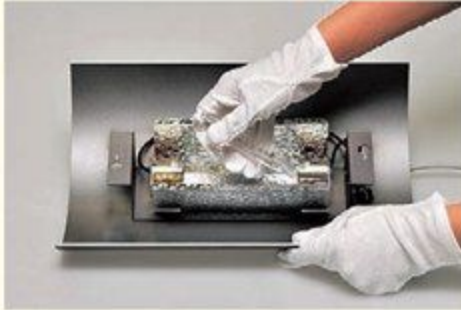
Wear cotton gloves to install the metal halide lamp to prevent contamination of the lamp with dirt and oil on the hands.
