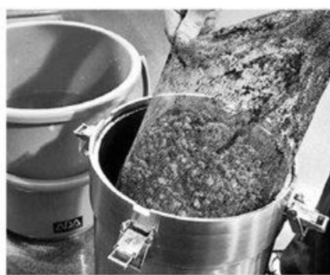
When using filter media in the net, sludge usually accumulates on the net.
