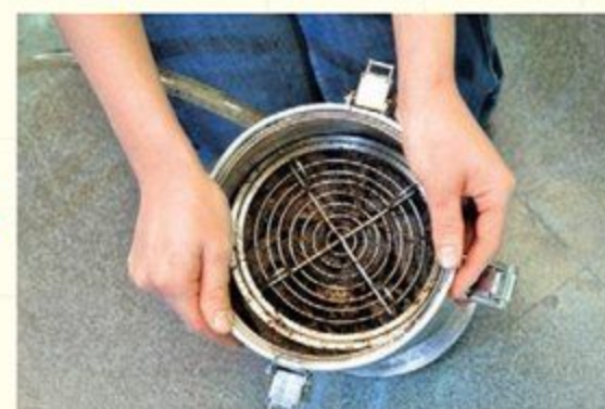
Even the top side of the filter media is quite dirty with sludge.
